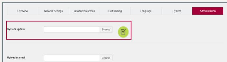
The software file is automatically transferred to the appropriate field. To complete the update, click on the button „Import“
