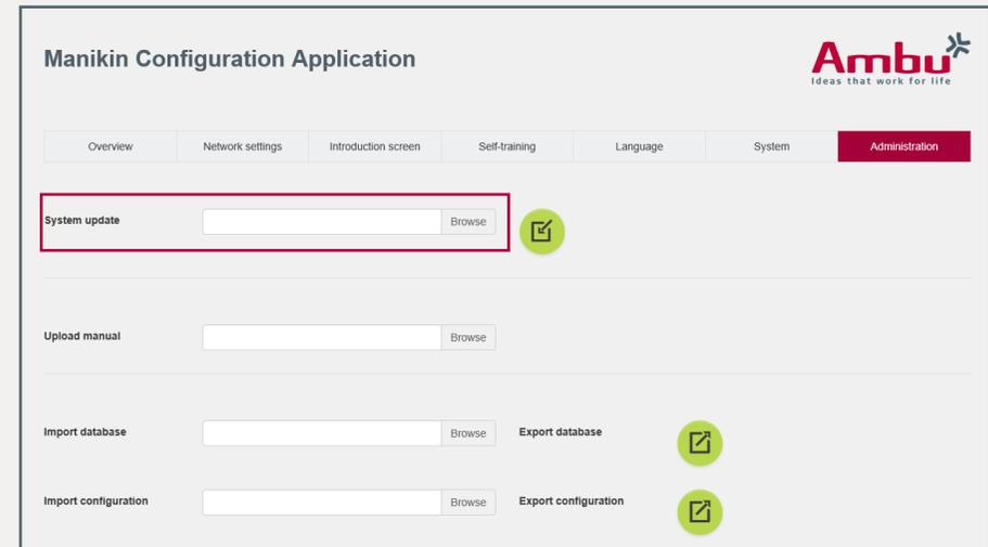
To load a new software update into the training device, open the appropriate file under „System Update“. By clicking on „Browse“ in the tab „System Update“ it is possible to search for the desired file.
